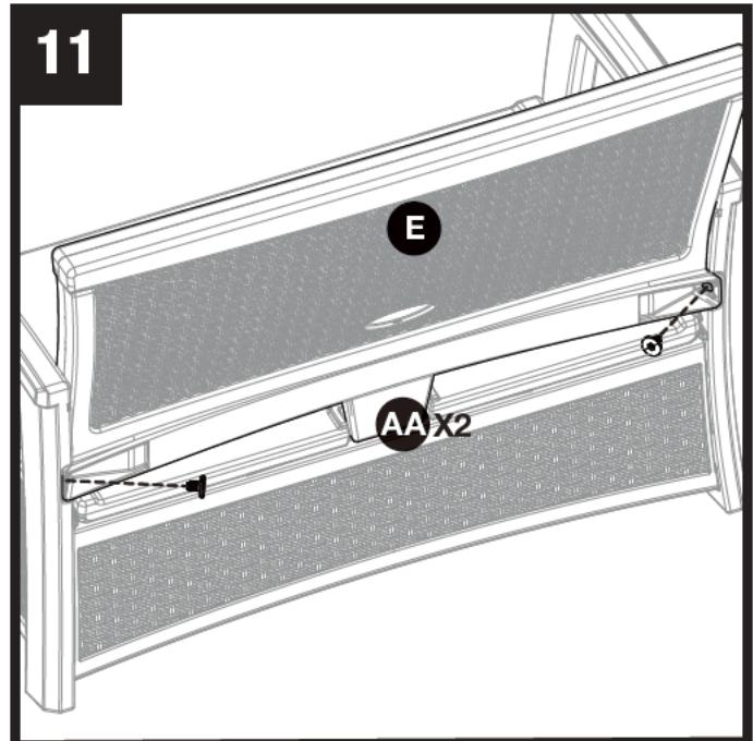
Attach back (E) to sides of loveseat using two easy bolts (AA).
