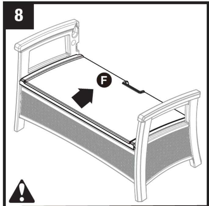
Lower seat (F) to base and insert large pegs in channel provided on each side panel of loveseat.
