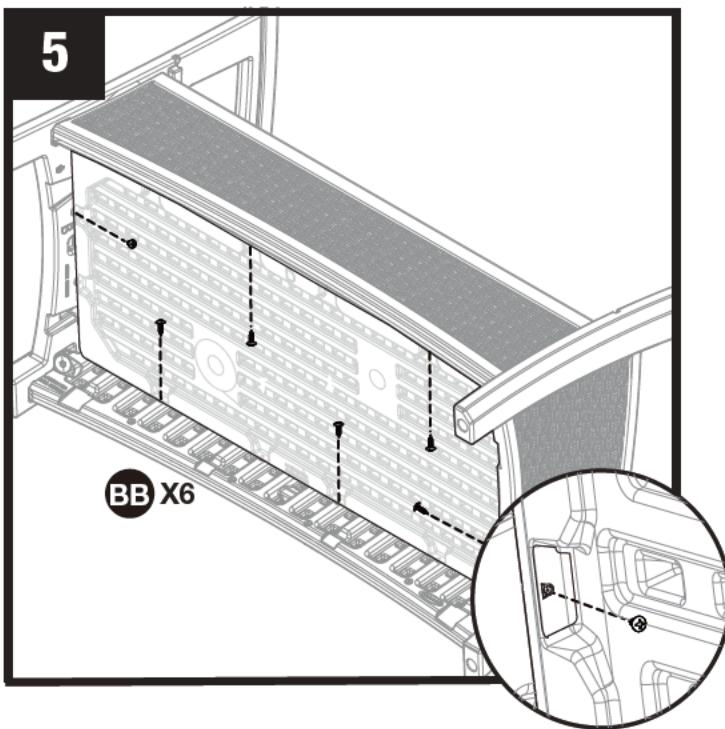
Attach bottom panel (D) using 6 screws (BB). Use force to pierce plastic. Turn loveseat right side up.
