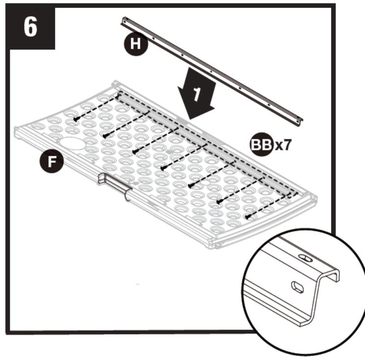
Attach bracket (H) to seat (F) using seven screws (BB). Oval holes on top are not used.
