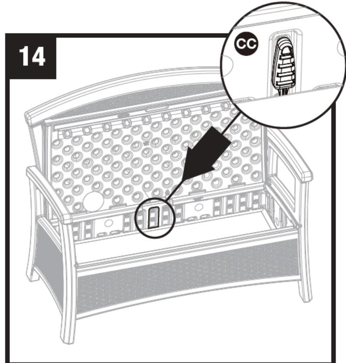
Insert plate (L) into back of loveseat. Peg on back of plate should insert into the center of the easy bolt. Snap in both sides until completely flat. Repeat other side.
