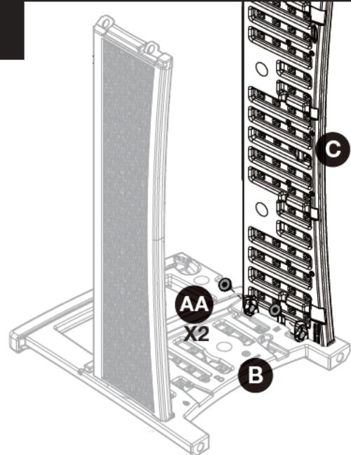
Lower panel (C) and insert into side panel (B).
