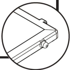
Place loveseat in proper orientation as shown above. Slide round pegs on bottom panel (D) into channel on left/right side of loveseat. To lock in place, push up hard until you hear a snap.
