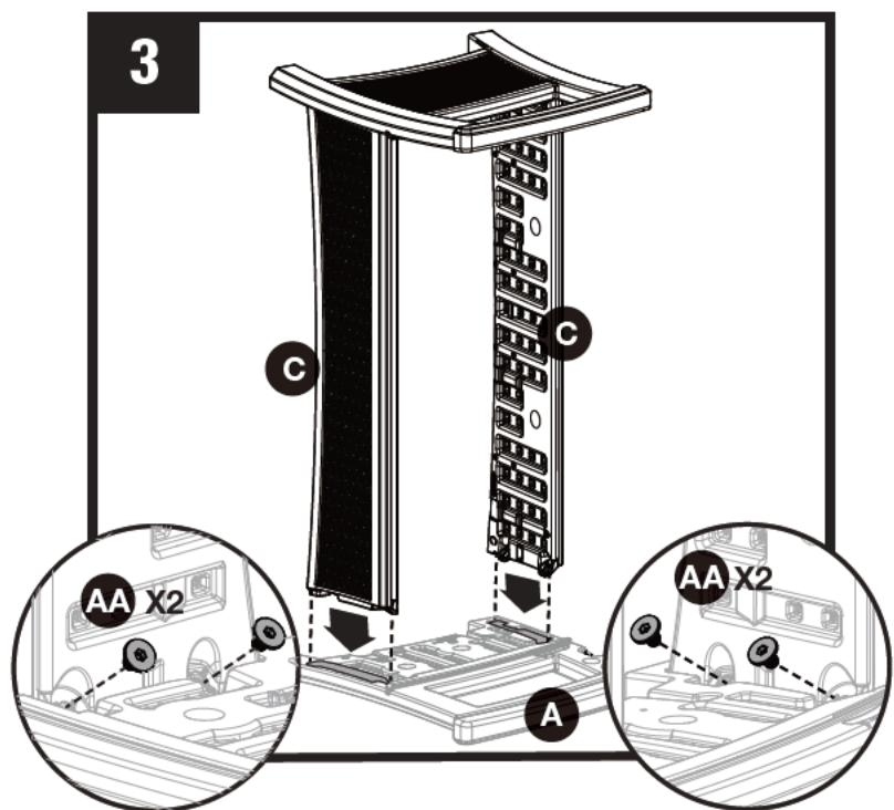
Lay side panel (A) on the ground. Lower assembly into side panel (A). Attach panel (C) to (A) with two easy bolts (AA). Repeat the other side.
